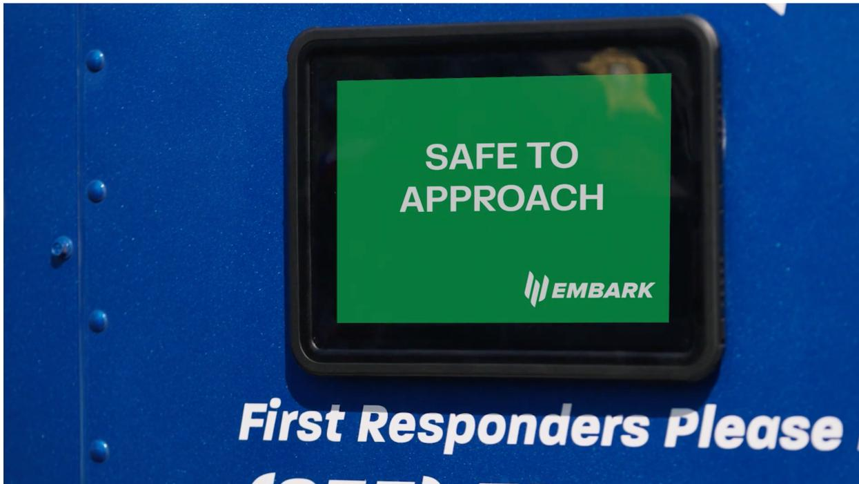
Example of status screen indicating autonomous truck is safe to approach after stopping on the highway shoulder.
