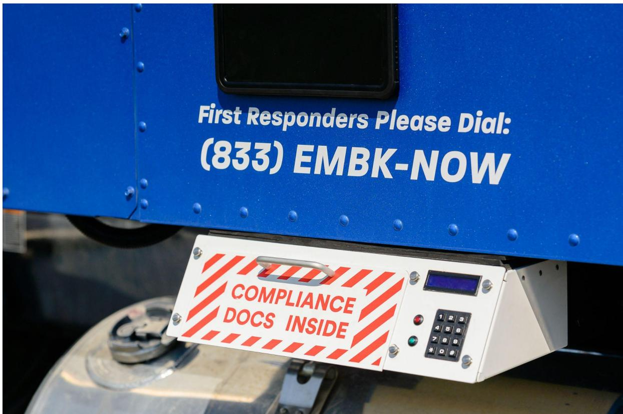
*Prototype LEO interaction features, including autonomous truck status display (top, currently off), support phone number decal, and compliance document lockbox.*
